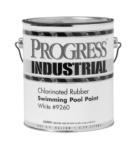
use on *unpainted* fiberglass pools. Covers approximately 400 sq. ft. per gallon on most surfaces. For best results, 2 thin layers are better than 1 thick layer. This product requires no thinning. If thinning is desired, use no more than 1 pint of xylene per gallon. Follow surface cleaning preparation and application instructions on the label. Apply with brush or roller. Clean tools immediately with xylene. Gallon.
